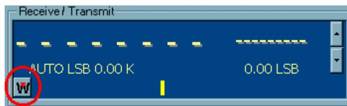
The Levels button
