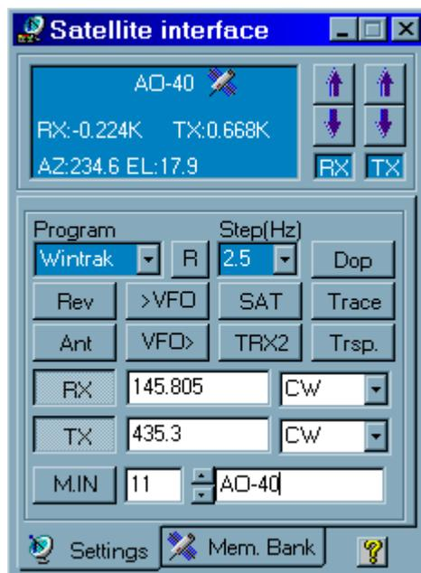
Once in Satellite mode, you can set up the Downlink or Uplink frequencies from the Edit/VFO (F2 key) or Edit/Split (F3 key) submenus. Setting up the satellite name is possible from the Edit/Info (Ctrl-I) submenu.
