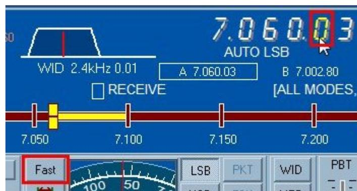
*Left/Right clicking a digit allows precise tuning OR engages a scanning depending on the state of the FAST button*
